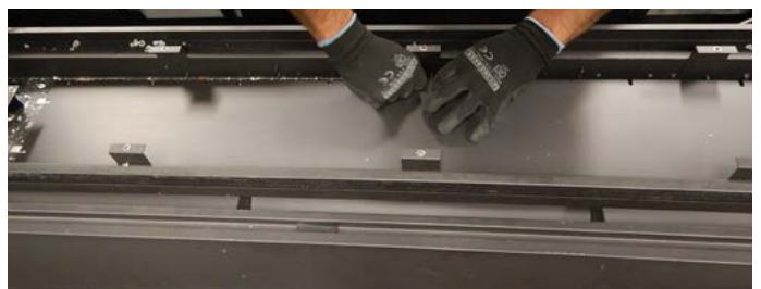
Figure 12.g Removing metal plate
