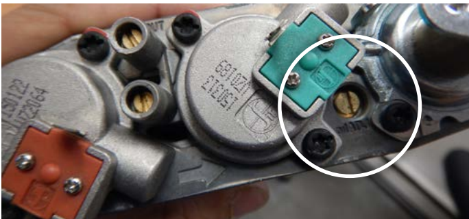
Figure 13.g Adjust pilot size
