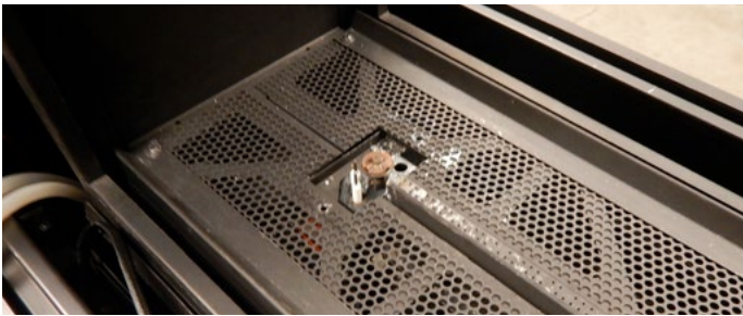
Figure 12. Removal of the pilot cover
