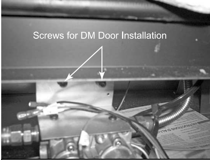
Figure 1 Pins & Screws for DM Door Installation - Reveal
