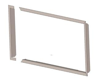
Ensure the all 4 corners of the trim kit are squared off. Before installation orient the trim so the notched section is on the bottom.
