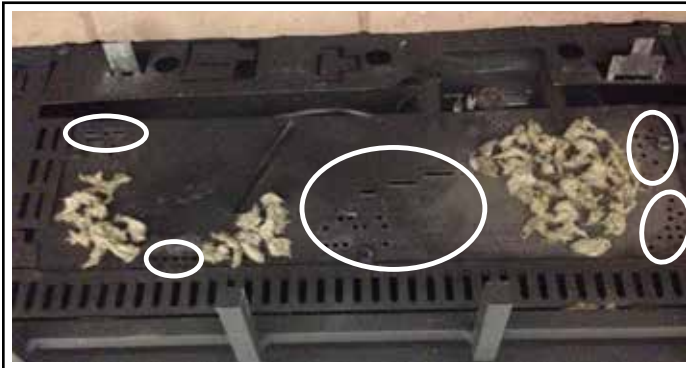
Figure 43 - Place glowing embers (rockwool)
