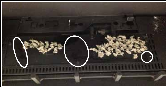
Figure H - Place glowing embers (rockwool)
