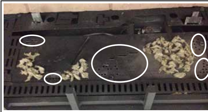
Figure 43 - Place glowing embers (rockwool)
