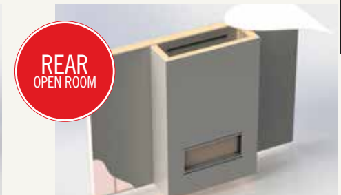
This style of enclosure includes an air outlet opening that will be built into the rear of the constructed enclosure above the appliance.
