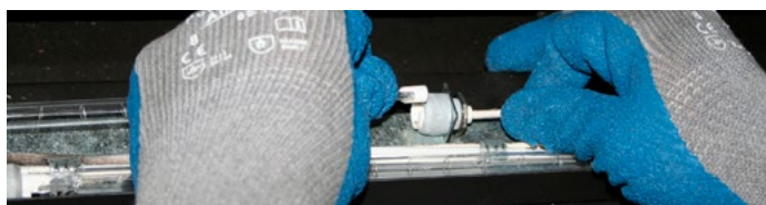
Figure 29.b Wear gloves when handling light bulbs. To remove a light bulb, pull connecting wire away from bulb and pull light bulb up. Replace with new light bulb.
