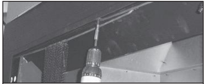
Figure 3.9 Removing the Screen Rods
