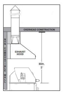
**Combustible Overhead Construction:** Exhaust hood required.
