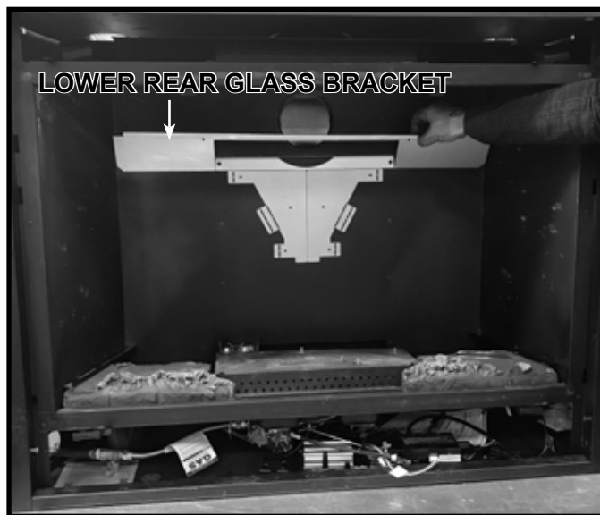
Figure 11.8 Removing Lower Rear Glass Bracket
