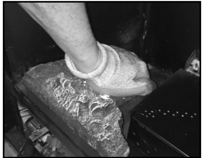
Figure 11.1 Press Left Hearth Firmly Into Place
